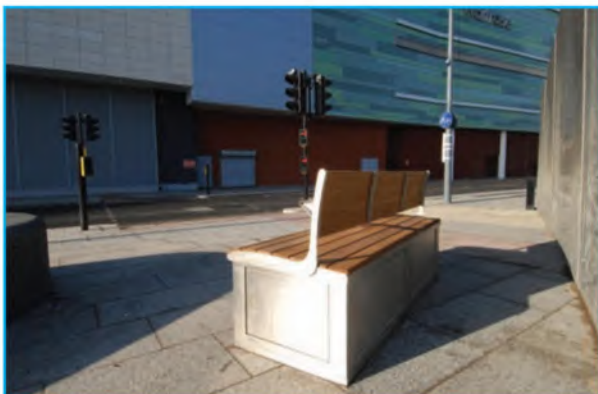
Bench containing traffic signal controller
