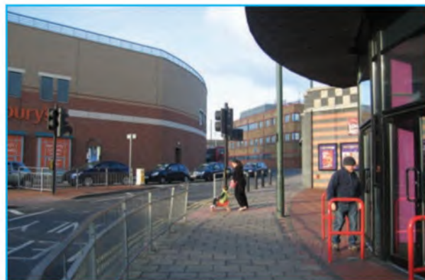
Segregated left turn lanes make pedestrian crossing movements more complex and slow, as well as adding to clutter.
