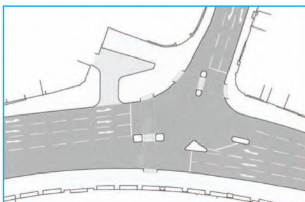
High Street Kensington - replacement of staggered crossing with straight over crossing at signalised junction.
