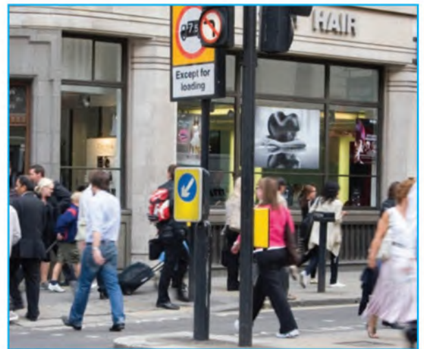
Sign to diagram 610 mounted on post. Note - yellow backing is not compulsory.
