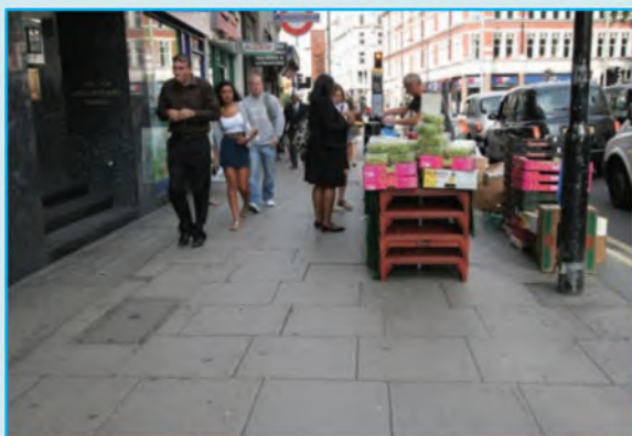
Street furniture and other clutter affecting footway capacity
