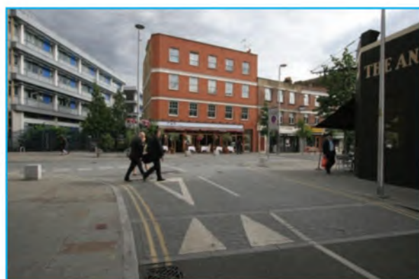
This junction has the Give Way marking (1003) and the approach triangle (1023) but no Give Way sign. It would have been possible to omit the approach triangle. Note also table to slow speeds and make pedestrian crossing easier.
